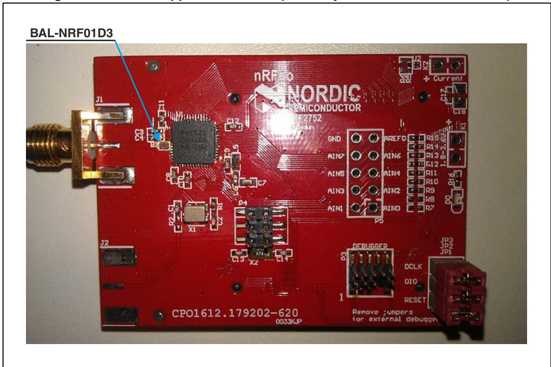
Figure 9. nRF2752 application board (courtesy of Nordic Semiconductor)
